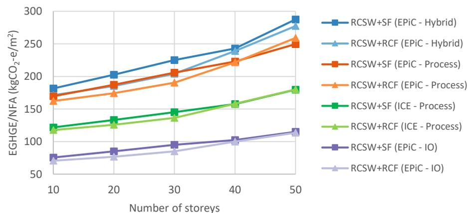
Figure 3 - Influence of life cycle inventory methods on the embodied greenhouse gas emissions per net floor area (EGHGE/NFA) of structural systems. Note: vertical axis starts at 50 kgCO<sub>2</sub>-e/m<sup>2</sup>.
