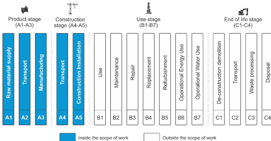
Figure 1 - Scope of the work according to EN 15978:2011
