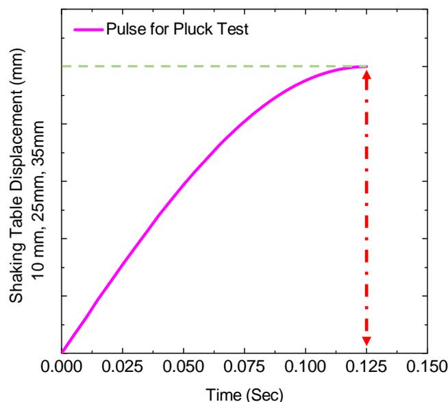
Figure 3 Pulse used for pluck test.
