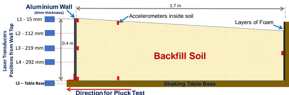
Figure 1 Details of scaled down retaining wall model.
