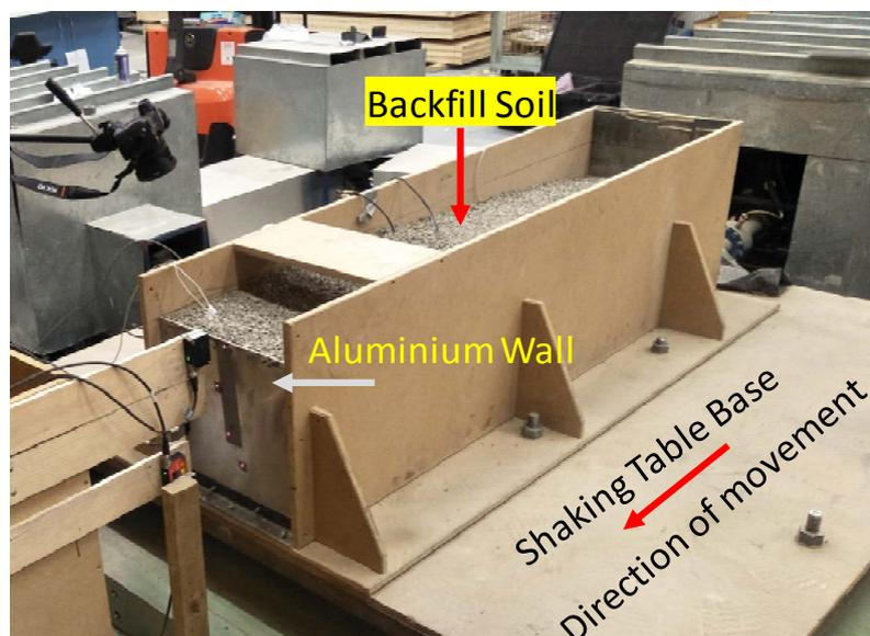
Figure 2 Experimental setup at The University of Melbourne.
