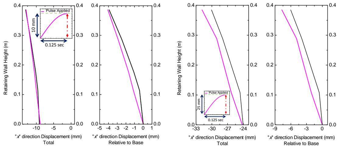
(a) “x” direction displacement along the wall height (bottom to top) for 10 mm amplitude pluck test. (b) “x” direction displacement along the wall height (bottom to top) for 25 mm amplitude pluck test.
