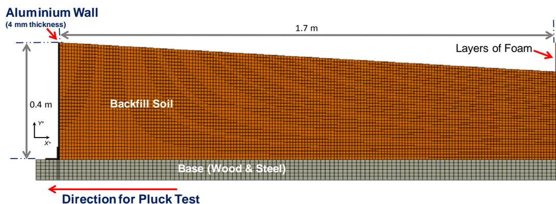
Figure 4 FE model of retaining wall in Abaqus.
